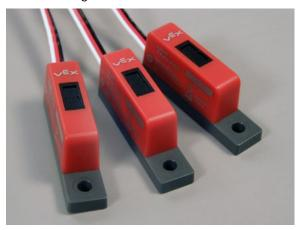
The Line Tracking Sensors can detect the basic colors of objects and surfaces by aiming directly at them at close range. They do so by illuminating a surface with its infrared LED and then measuring how much light is reflected back.
