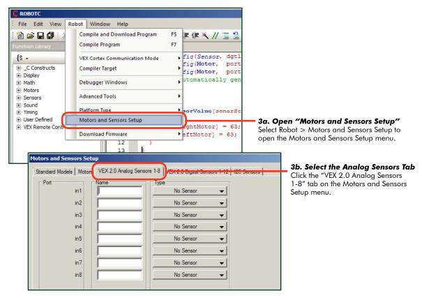
**4.** Use the Motors and Sensors Setup menu to name the in2 sensor "centerSensor", then select "Line Follower" as its type. Note that we only need to use one of the three line tracking sensors for the Forward until Dark behavior. The center sensor is a logical choice, but any of the three sensors would work.
