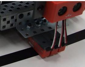
Light-colored surfaces, like the bright white table, reflect a large amount of the light, and produce a **low** sensor reading. Dark-colored surfaces, like the strip of black electrical tape, reflect very little light, and produce a **high** sensor reading.
