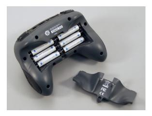
1b. Install Batteries in the VEXnet Remote Control Remove the battery cover plate on the remote control. Install 6 AAA batteries, and replace the battery cover plate. Do not power the remote control ON.
