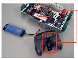
6. VEXnet USB Keys Insert VEXnet USB Keys into the VEXnet Remote Control and Cortex.
