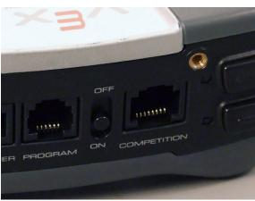
7b. Turn the VEXnet Remote Control ON
