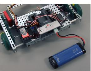
**1a.** Connect a Battery to the Cortex Connect a 7.2V robot battery to the Cortex, but do not power it ON.
