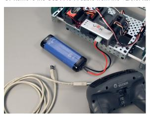
6. Insert VEXnet USB Keys into both the VEXnet Remote Control and Cortex.
