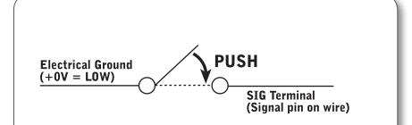
Signal pin is HIGH when switch is open Pushing switch brings the signal pin voltage to LOW
