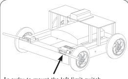
In order to mount the left limit switch, position it upside down using spacers to support the area where the screws are applied.
