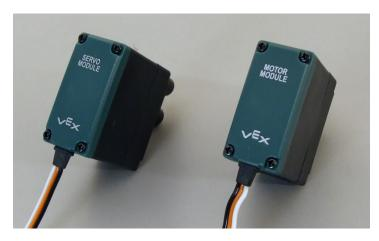
The only differences in appearance between the VEX Servo and Motor Modules are their labels on the back, but the two should not be confused. When a Motor Module is set equal to a value, it uses that value as a power setting and starts spinning its shaft in continuous rotations. When a Servo Module is set equal to a value, however, it uses that value to rotate its shaft to a position and hold it there.
