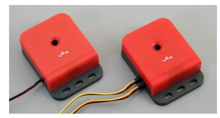
The upgraded Quadrature Shaft Encoder includes a second optical sensor which allows the sensor to detect if the internal disk is spinning clockwise or counterclockwise and increases the resolution to 360 counts per revolution (2 count intervals). Two output channels (wires) are needed to transmit its sensor data to the Vex.
